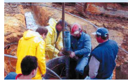
The 'Optical Caterpillar' is sunk into its hole
