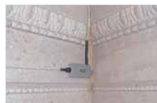
Detail of an optical strand on angle.
