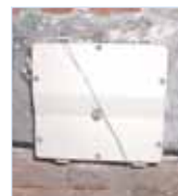
Cabled X-Trigger as a crack meter.
