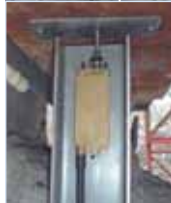
OSMOS-WIMS installed on the Viaduct of Murrthal (See p4) Above, one of the WIMS sensors.
