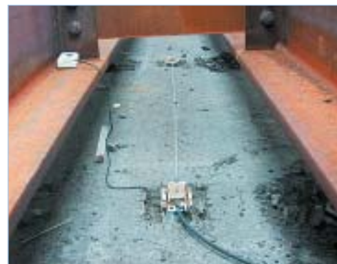
Optical strand on the upper face of one span
