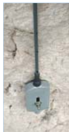
Optical strand in flexible steel sheath - deep anchorage with high-resistant resin
