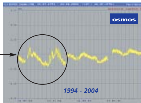
Measurements taken by one of the optical strands on the tympanum over a period of 10 years. The first 2 years of observation stand out clearly from the following years, due to the placement of steel arches and shotcrete on arch 28
