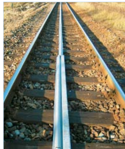
OSMOS sinkhole watcher over a length of 800 m overall view at the beginning of the monitoring
