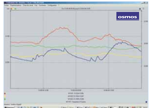
Daily measurements combining deformation and inclination of the building
