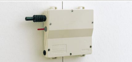
Top photo: X-Trigger as a fissure width monitor, wired; Bottom left photo: X-Trigger as a sleeping alarm fuse; Bottom right photo: X-Trigger as a probe.
