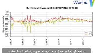
and flexion of the church buttresses. By running a dynamic analysis, we can assess the impact on the structure and confirm if it has returned to its balanced state.
