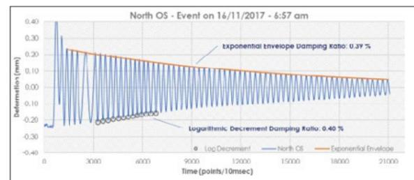
Calculation of damping coefficients
