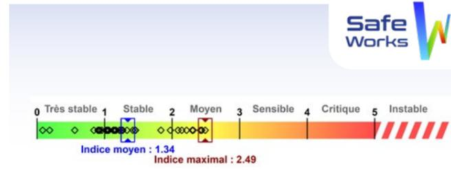
The result is a single, overall score for each sensor. The usual scale is from 0 (stable) to 5 (unstable), appearing in the form of the letters A to F in the SAFE Works interface.
