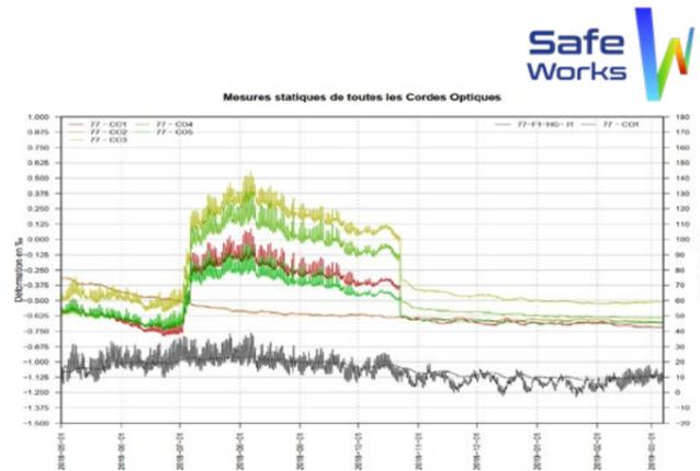
When a pipe bursts, tensioning is observed in a load-bearing wall. That tensioning is proportional to the distance of each Optical Strand from the fault. Later, after reinforcements have been applied, we can see the return to normal operations.
