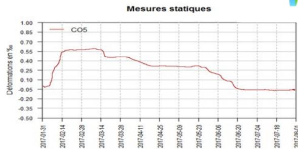
Over the course of several months, we have observed separation of stone blocks on each pillar. The progressive return to its initial balanced state was observed over this time period.
