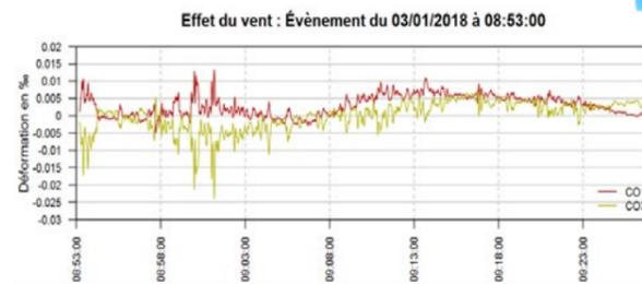
During bouts of strong wind, we have observed a tightening and flexion of the church buttresses. By running a dynamic analysis, we can assess the impact on the structure and confirm if it has returned to its balanced state.
