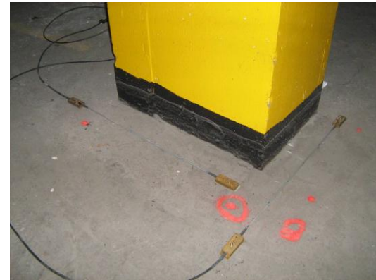
Optical Strand locations to measure longitudinal and transversal deformations of the slab
